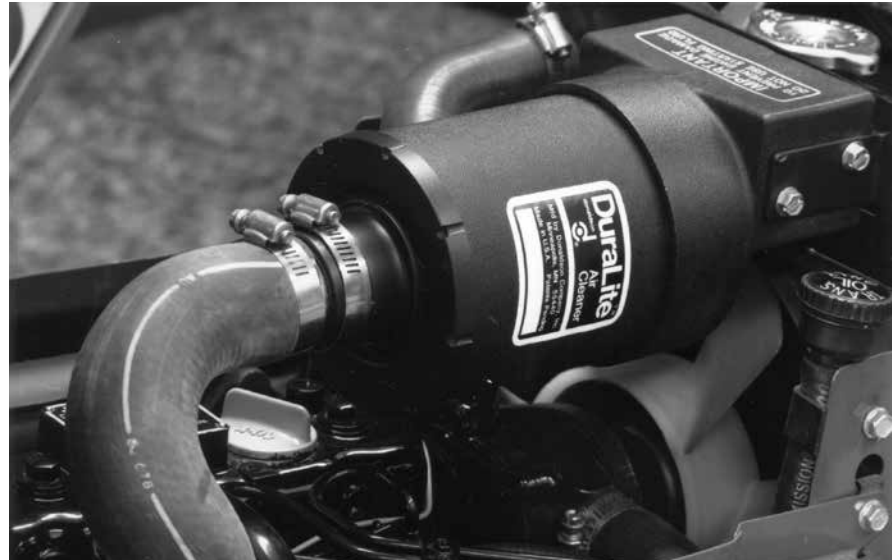
DuraLite™ Air Cleaners — sturdy, one-piece, and disposable — are designed to withstand the high pulsation of small engines such as the ones shown here. They are easy to maintain because there are no service parts. When the filter is full, simply throw it away.
